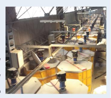
In summary the EMF Motor solution continuously produces very high torque at really low speed. The speed and torque is maintained accurately even in open loop configuration. The motor is extremely efficient resulting in minimal power consumption. The EMF Motor requires no gearbox, no maintenance and no additional cooling. EMF Motor works with ceramic product manufacturers to provide the most reliable and efficient production solution and enable the highest level of glaze product quality.
