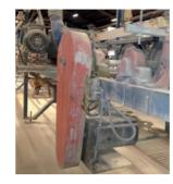
**Coveyor motor** for waterfall application of glazes and engobes
